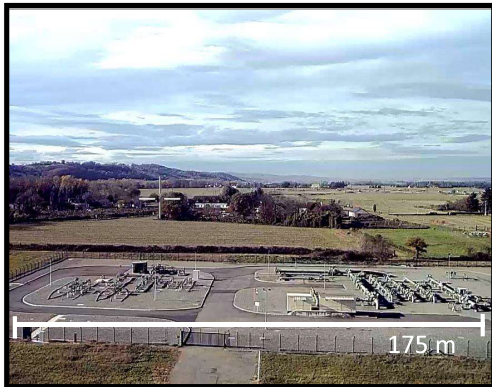
LARGE SURVEILLANCE AREA Average flying height of 25 - 30 m with a 60° field of view Operational over more than 300 ha
