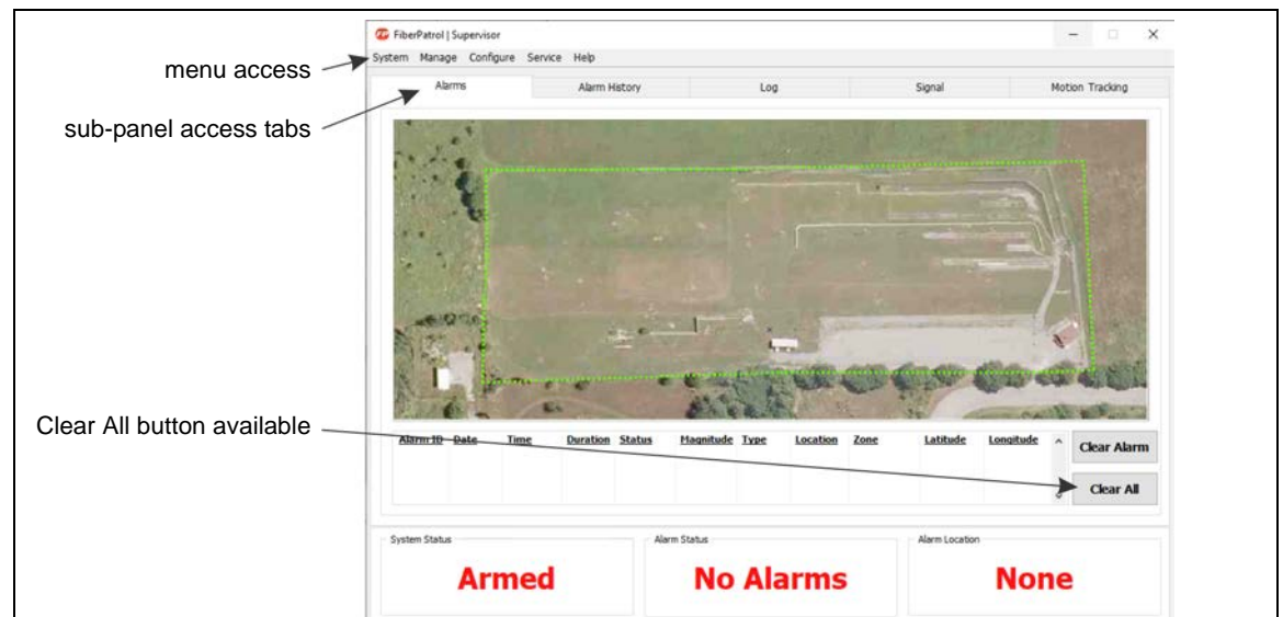
Figure 142: FiberPatrol Supervisor access level display
