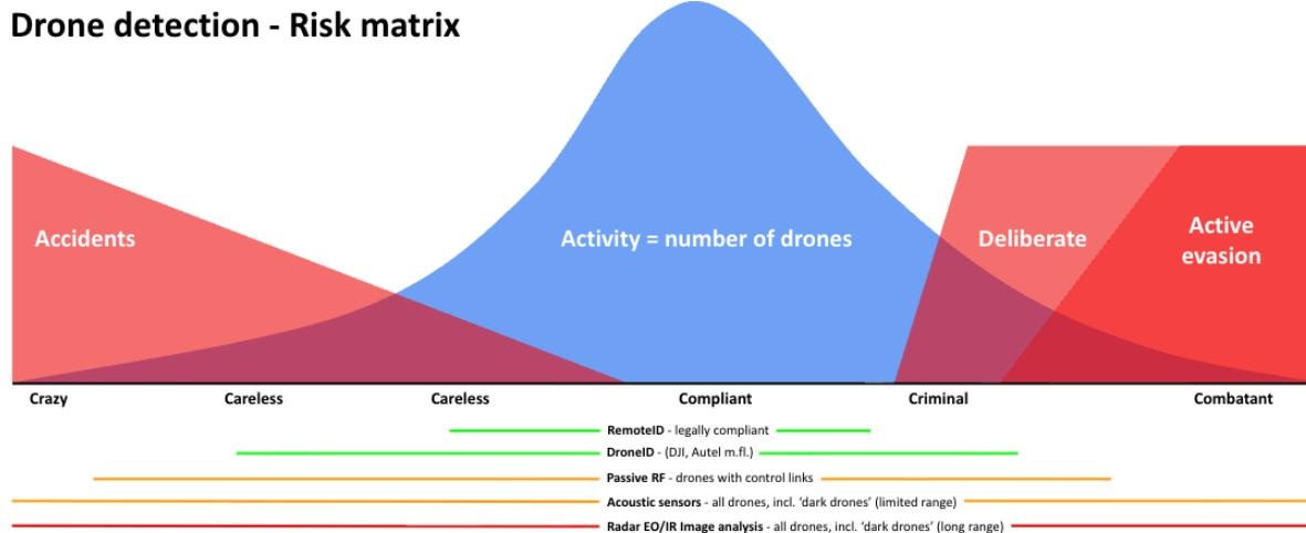
**Note.** As the illustration shows, detecting autonomous drones requires acoustic sensors or radar.
