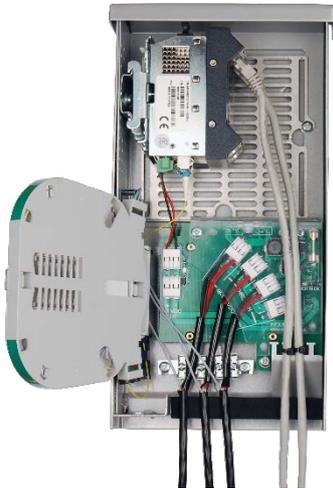
This instruction contains information how to terminate Hybrid Micro cable to Termination Box HNCD 520 232. The Termination Box is a part of Hexatronic Powered Fiber Network and shall only be powered by that system. It is designed to be mounted in a weather protected area on wall or in suitable cabinet.
