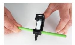
For duct version, make a slit along the cable from the notch to the end using the LDK 19503 (note that the blade with rounded edge shall be used). For In-Outdoor version slightly bend the cable to make the sheath to break in the cutted area
