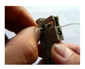
Carefully break the tube at the notch and pull off the tube.
