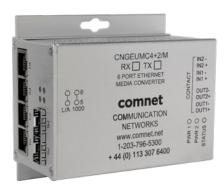
The ComNet CNGEUMC4+2(TX,RX)/M unidirectional media converter with Link Guardian limits network traffic to one way communication between source and destination networks preventing cybersecurity attacks from a non-secured entry point in the network from reaching a secured part of the network. The CNGEUMC4+2(TX,RX)/M provides four 10/100/1000Base-T(X) copper ports and two 1000base-FX SFP ports.
