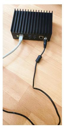
Connect the U-Alarm box to the Ethernet network using the primary Ethernet port of the device.
